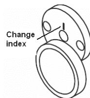
Key hole maximum diameter must be 12mm. Fit escutcheon on outside making sure that change index is properly aligned (change index) according to lock handing.
